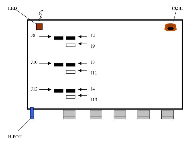
Opening the J2, J3 and J4 pins will remove the 75 ohm termination for each color. This setting allows users to connect a cable such as the **IN9041** to the input and utilize a local monitor. Please note that if there is no local monitor and the jumper pins are set to this position, there will be unnecessary "blooming" or overdriving of the other four outputs.
